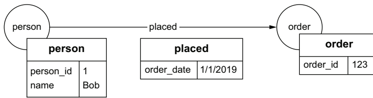
Figure 7.10 Order-processing system graph from chapter 5 with only the order_date on the placed edge
